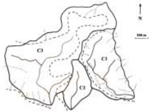
Figure 20.3. A map of the Bukit Berembun C1, C2 and C3 catchments in Peninsular Malaysia, showing catchment divides (wide, solid lines), streams (narrow, solid lines), timber haulage roads (broken lines) and skidder trails (dotted lines).
